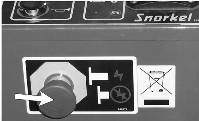
**Figure 2.1 - Platform Control Box Emergency Stop Switch**
