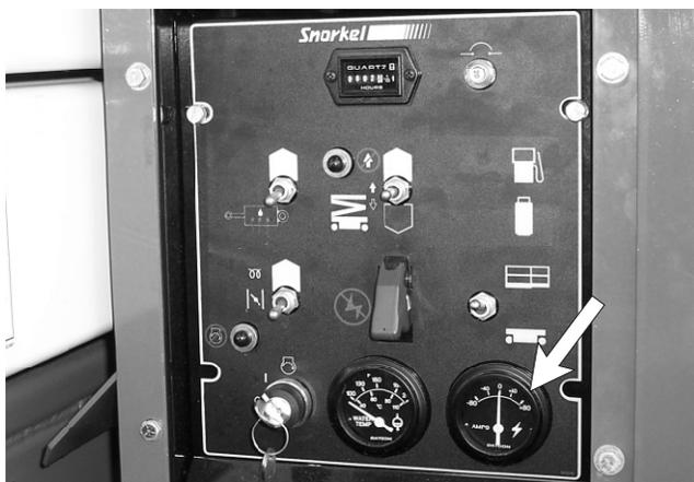
**Figure 4.2 - Ammeter Gauge**
