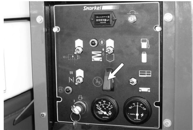
**Figure 8.1 - Emergency Stop Switch at Ground Control Box**
