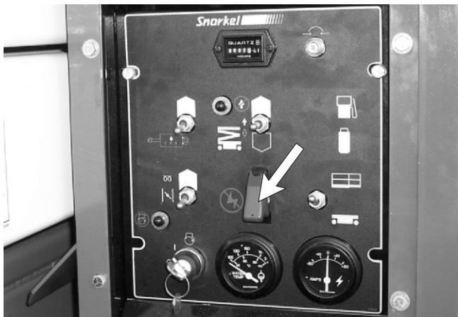
Figure 9.2 - Ground Control Box Emergency Stop Switch
