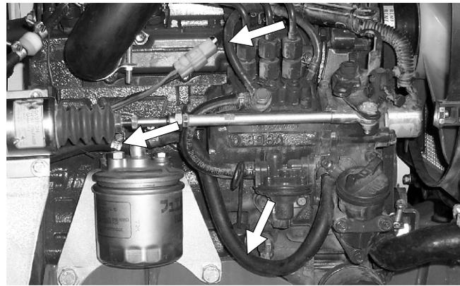
**Figure 7.4 - Fuel Leaks in Hoses & Joints**
