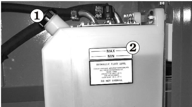
Figure 7.13 - Hydraulic Oil Tank
