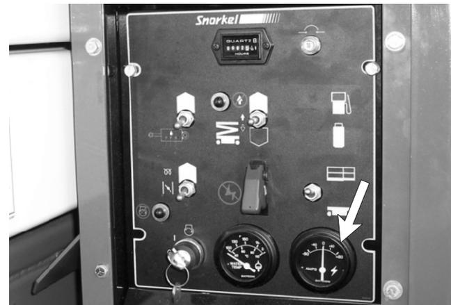
**Figure 7.23 - Ammeter Gauge**
