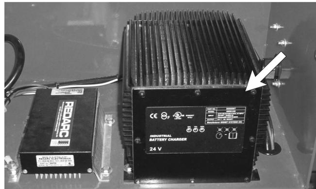
Figure 11.8 - On-Board Battery Charger
