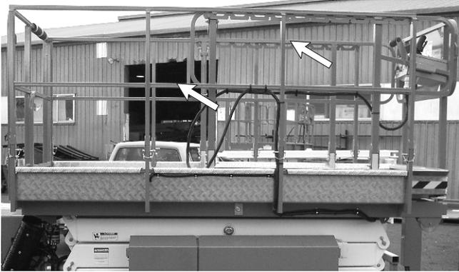
**Figure 7.20 - Guardrails**
