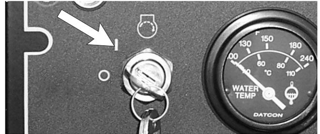
**Figure 11.3 - Start Switch, Ground**
