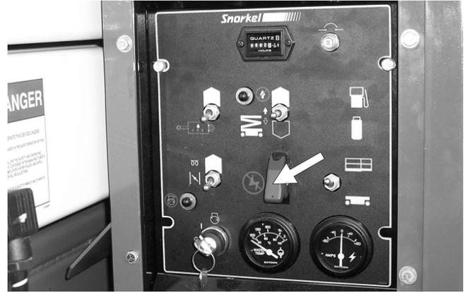
**Figure 2.2 - Ground Control Box Emergency Stop Switch**
